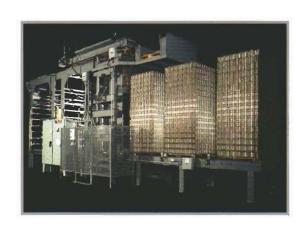
sheet clamps release and the sheet is removed and stacked in a storage bin. The lift will raise the load to repeat the cycle until the pallet is emptied. The lift lowers and the empty pallet is conveyed out of the lift station to a pallet stacker which will typically hold 8 pallets.
